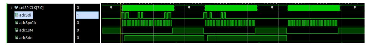
Write xD814000b, 32 spi clks using mode 0 1 us from falling edge of CONV/~CS to first SPI CLK
