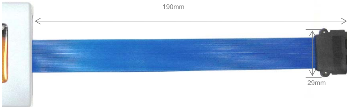
Figure 6 - Target Interface Cable (top view)
