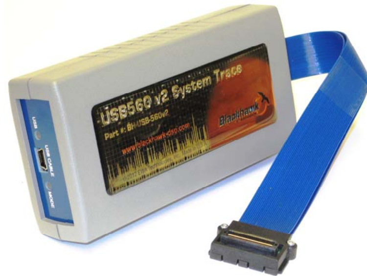
Figure 1 - BH560v2 Pod and Target Cable
