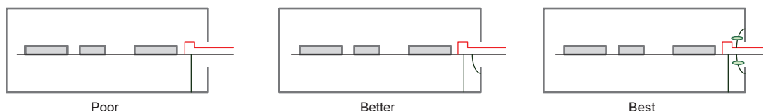
Figure 14. Enclosure Cable Considerations
