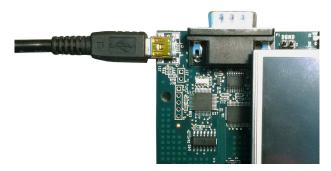
As soon as the USB cable connects to your host PC, Windows should automatically recognize that new hardware has been connected and install the necessary drivers. Power on your OMAP-L138 eXperimenter Kit and continue with the next section.
