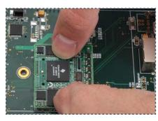
Connect OMAP-L138 SOM (use outline on baseboard for positioning), press straight down over connectors
