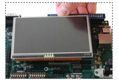
Connect 4.3" LCD, remove protective plastic covering
