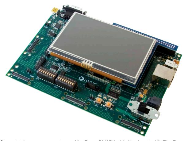
Congratulations on your purchase of the Zoom OMAP-L138 experimenter Kit. This Zoom Development Kit provides a product-ready hardware and software platform for evaluating the functionality of the Texas Instruments (TI) OMAP-L138 processor and the Logic PD System on Module (SOM).
