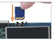
Insert Linux SD card (slot on bottom of baseboard)
