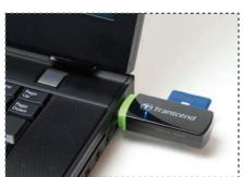
Remove SD card and insert it into included USB SD card reader: connect USB SD card reader to host PC
