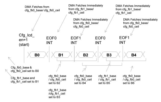
B0, B1, and B2 can be black frames. A video framebuffer must be available every EOF interrupt. On the first EOF0 ISR, configure fb0 (only if B2 is not a Black frame) and fb1. Then, subsequent EOF1 ISRs update fb0 and EOF0 ISRs update fb1.
