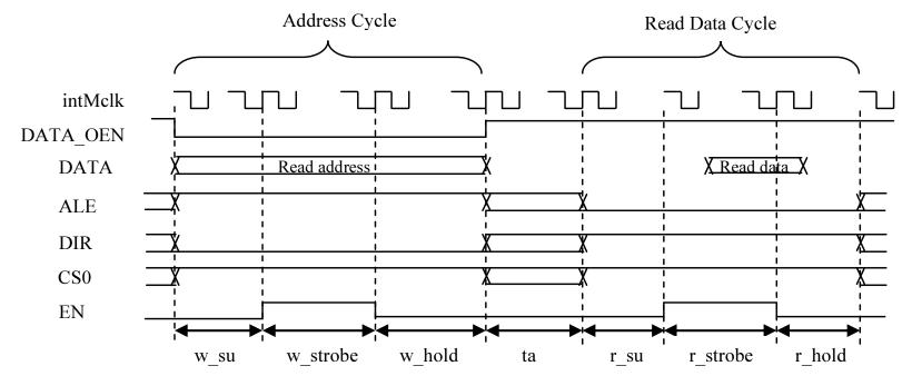
The address is loaded into the external latch when the CPU writes a value to LIDD\_CSx\_ADDR. ALE is active and DIR is low (write).
