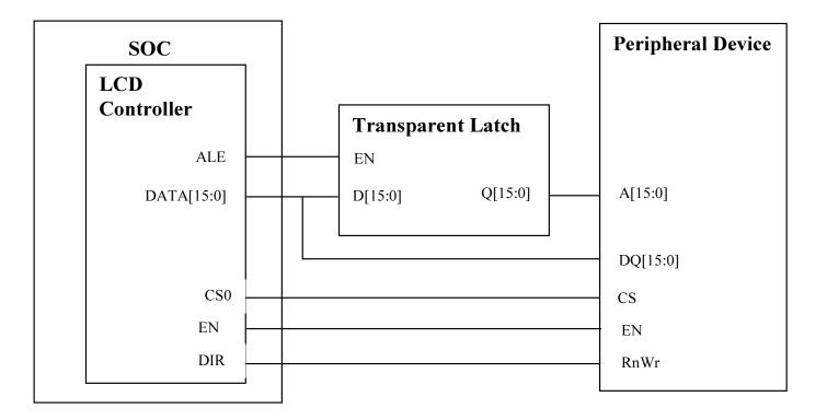
The Motorola 68k mode uses a shared 16-bit address/data bus. The address is sent first, latched externally, and then data is sent to complete the bus transaction. The external logic required for using the shared address/data bus is shown here.
