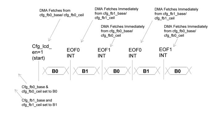
Two frames, B0 and B1, are needed at the start. However, B0 can be a black frame (the Host creates a black frame in DDR). In this case, a video display framebuffer must be available at the start and for every ISR.
