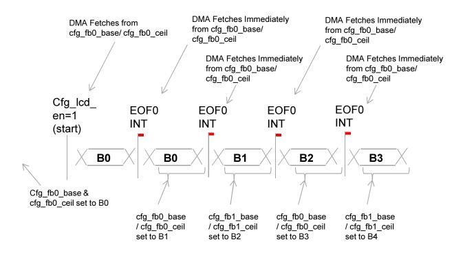
For Use Case 4, there is a Race Condition in which the Host CPU must not update cfg\_fb0\_base and cfg\_fb0\_ceil until after the DMA engine has read the values in the CPU Keep-out regions shown in Red. Practically, though, the interrupt latency for the CPU is expected to be long enough to ensure that the configuration registers cannot change in the Keep-out region. The ISR must update the pointers before the next interrupt, though.
