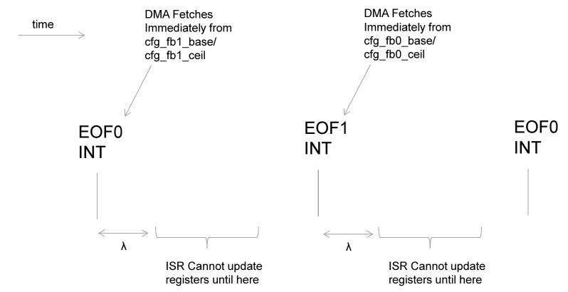
After an EOF0 or EOF1 interrupt, it takes a certain latency  $\lambda$  before the ISR can set cfg\_fb0\_base, cfg\_fb0\_ceil, cfg\_fb1\_base, and cfg\_fb1\_ceil.
