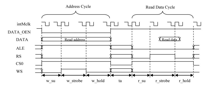
The address is loaded into the external latch when the CPU writes a value to LIDD\_CSx\_ADDR. This CPU write activates ALE for the transaction.
