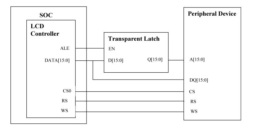
The Intel interface mode uses a shared 16-bit address/data bus. The address is sent first, latched externally, and then data is sent to complete the bus transaction.
