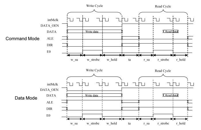
The Hitachi style bus model is shown here. intMclk is the internal bus clock and is shown for reference only. ALE is low during the transaction if the Host is reading or writing a command. A command is initiated by writing to the LIDD\_CSx\_ADDR register. DIR determines whether the bus transaction is a read or a write. E0, shown to be active high, is the data strobe for device 0. For a read, external read data is expected to be ready the intMCLK cycle just before E0 goes inactive
