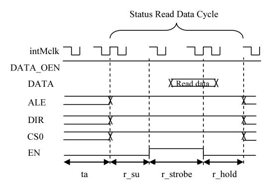
The Motorola bus allows a transaction to read a single status vector from the target peripheral. This status read transaction does not require an address, since it returns only a single vector. The CPU initiates a status read transaction when it reads from the LIDD\_CSx\_ADDR register. ALE is active, signaling a read-status transaction. CS0 is active. EN is used as a strobe signal to the external device. External read data is expected to be ready the intMCLK cycle just before EN goes inactive.
