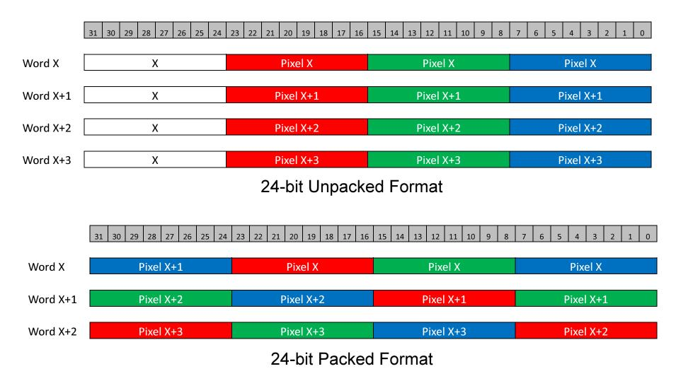
Using packed format reduces frame buffer size by 25%
