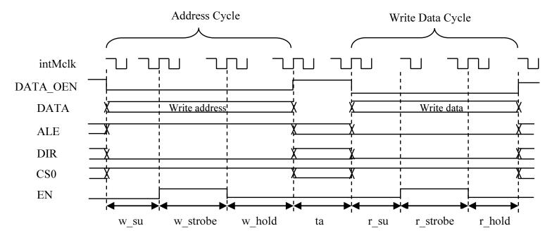
Signals are shown active high. DIR is shown to be high for a Read and low for a Write.
