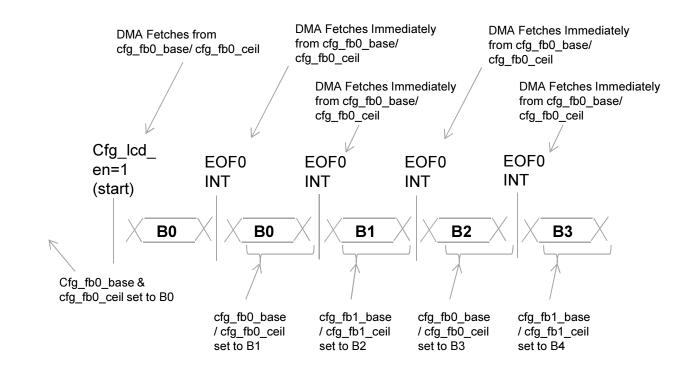
B0 can be a black frame. A video framebuffer must be available every EOF0 interrupt, which is used to trigger the ISR that updates cfg\_fb0\_base and cfg\_fb0\_ceil. This scenario is very similar to Use Case 1, which uses Ping Pong Buffers.
