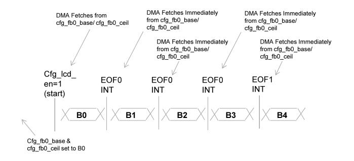
The Single Buffer Usage Model was designed for the case where the framebuffer pointers are static. A fixed display buffer in DDR has new frames copied into it by the CPU or DMA.
