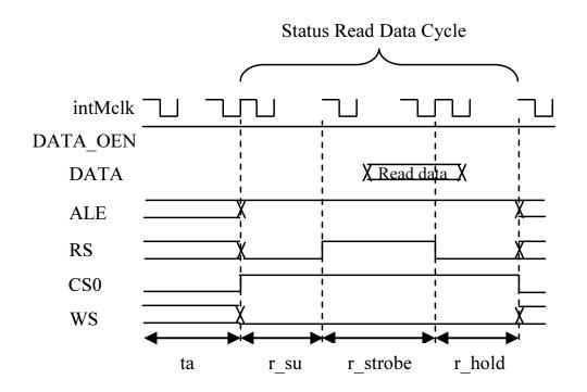
The Intel bus allows a transaction to read a single status vector from the target peripheral. This status read transaction does not require an address, since it returns only a single vector. The CPU initiates a status read transaction when it reads from the LIDD\_CSx\_ADDR register. ALE is active, signaling a read-status transaction. CS0 is active. RS is used as a strobe signal to the external device. External read data is expected to be ready the intMCLK cycle just before RS goes inactive.
