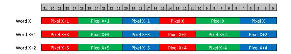
The frame buffer size for 16-bit is 50% less than the unpacked 24-bit.
