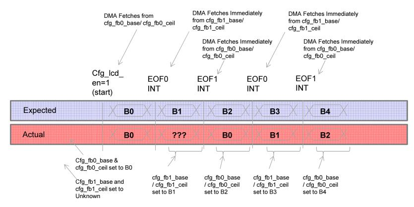
The intent is to try and set the upcoming framebuffer location at each EOF0/EOF1 ISR with the expected result shown in Blue.
