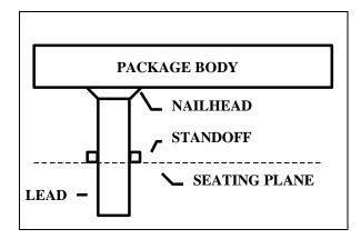
Due to normal variations in the solder dip process, some devices will have gold plate exposed on the nail-head, some will not, and some devices will have both gold and soldered nail-heads. As illustrated on the left, the nail-head is above the seating plane of the device therefore the presence or absence of solder on the nail-head is not an issue.
