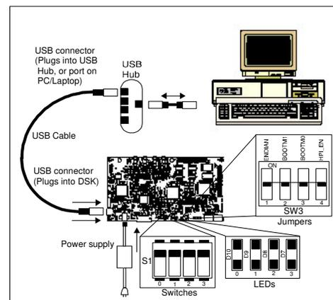
6. Make sure your DSK CD-ROM is installed in your CD-ROM drive. Now connect the DSK to your PC using the included USB. After few seconds Windows will launch its "Add New Hardware Wizard" and prompt for the location of the DSK drivers.
