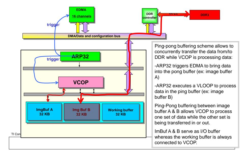
Due to size of image buffer, VCOP can only operate on 32 kb of data at a time. The original image is divided in blocks. To process the entire image by VCOP, every block of the image is transferred from DDR to image buffer, processed by the VCOP and then transferred back to DDR.
