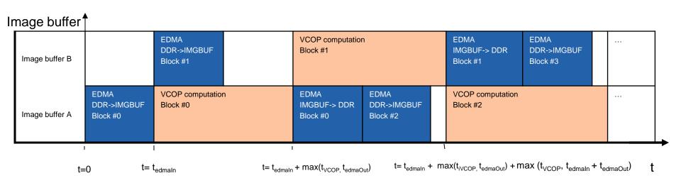
Concurrent processing Graph Total execution time for one block is  $t = max (t_{VCOP}, t_{edmaIn} + t_{edmaOut})$
