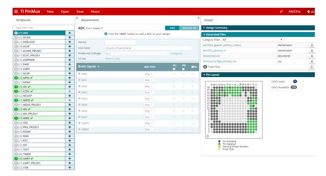
Add and remove peripheral instances and select the appropriate use cases required for development based on the application platform requirements and resolve all conflicts.
