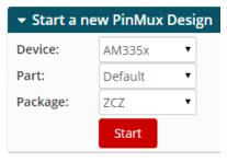
Navigate to \${PDK\_INSTALL\_DIR}\packages\ti\starterware\tools\pinmux\_config\am335x and Load beaglebone\_black\_config
