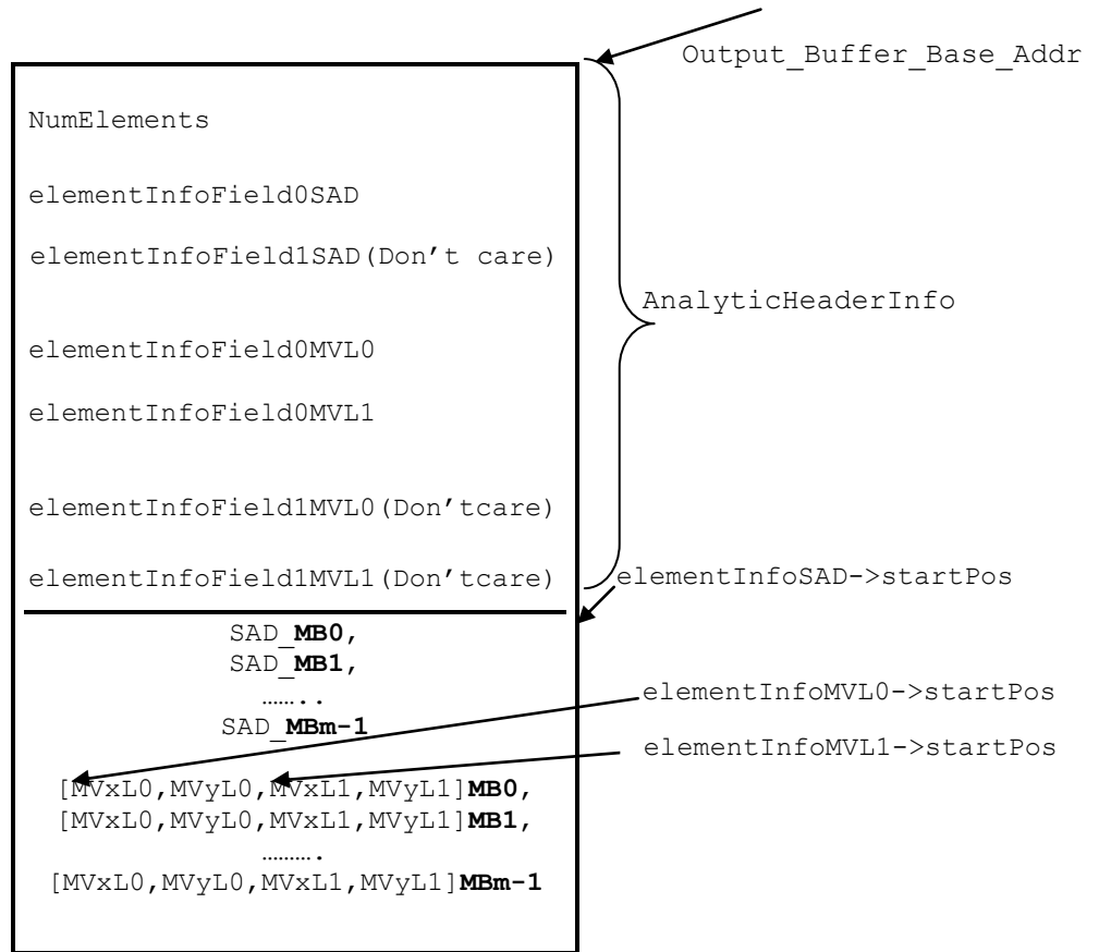
Figure D-5. MV and SAD data dump by codec in case of progressive B frames.
