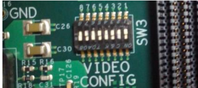
VIDEO CONFIG switch settings (SW3 on TDA2xx Vision Application Board (set for Ov10635 in Original version of CPLD))
