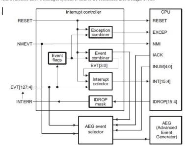
The figure below shows a logical representation of the Event Combiner in the Keystone CorePac. The 124 system events are divided into 4 groups, as shown in the figure below. The Event Combiner logic has the capability of grouping multiple event inputs to 4 possible event outputs, EVT[3:0]. These outputs are then provided as inputs to the interrupt selector and treated as additional system events. This is illustrated in the figure above [2]
