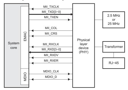
Figure 2. Ethernet Configuration—MII Connections
