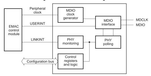
Figure 10. MDIO Module Block Diagram
