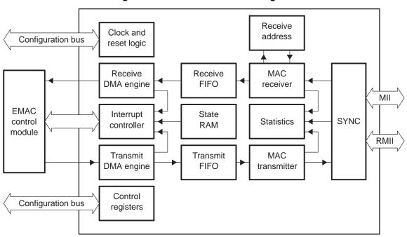
Figure 11. EMAC Module Block Diagram
