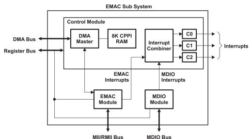
Figure 1. EMAC and MDIO Block Diagram
