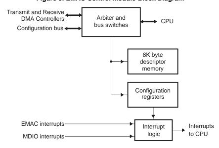
Figure 9. EMAC Control Module Block Diagram
