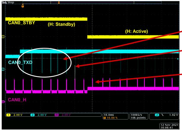
AM3356 output the unexpected data, but, it does not appear on CAN BUS because of Standby state.
