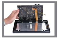
Position the IDK board close to the LCD screen and connect the LCD cable to the IDK board using connector J16. The cable should be connected with the contacts facing away from the IDK (up). Ensure the connector is secure by pressing down on the black flap.
