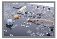
Connect the touch cable to the IDK board using connector J17 on the back side of the board. Make sure the connector is in the open position with the black portion slid outwards. Insert the plain end of the touch cable into the connector with the contacts facing away from the IDK (up). Close the connector to secure the connection.
