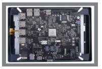
Mount the IDK on the LCD screen so that the screws on the LCD assembly fit through the holes on the PCB and attach standoffs to secure the board. Note that two standoffs must be attached if the camera module will be used. Tighten standoffs only to finger tightness; overtightening may loosen the assembly from the display frame.
