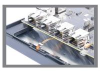
Connect the touch cable to the LCD screen using the connector on the end of the cable. The connector is opened and closed using the black flap.
