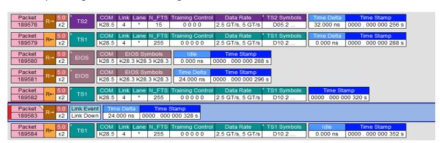
IDT switch link goes down at packet and 190566 and downgrade to Gen1.
