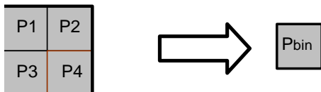
Figure 9-2. Color binning (color_en=1)
