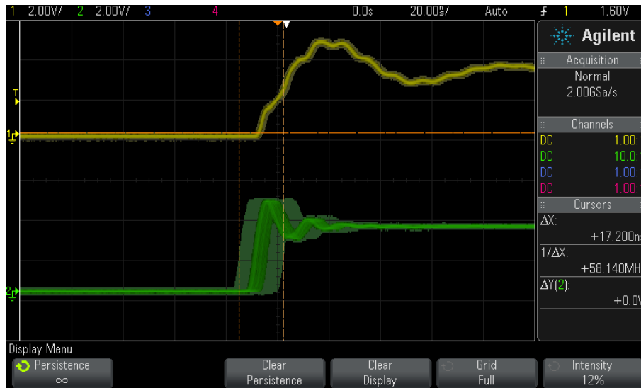
Topology (2) oscilloscope capture showing Sync Pulse jitter measurement between two K2G ICE boards
