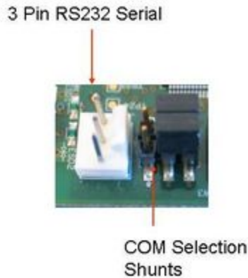
Figure 9 - Shunts for Serial Port
