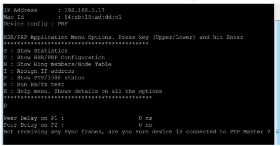
The menu shows the current offset from master, line/peer delay (for both ports) and current time (UTC offset).
