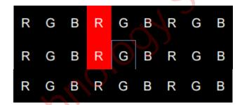
Two adjacent dots (bevel direction): Use the bright spot illustration as an example to demonstrate two consecutive dots in the bevel direction.
