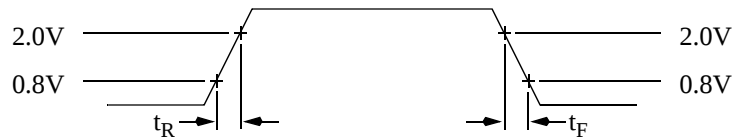
FIGURE 7. Input/Output Valid Level for AC Measurements
