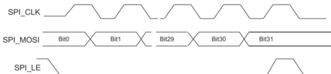
Figure 5.7: SPI access from FPGA to CDCE62005 (WRITE)
