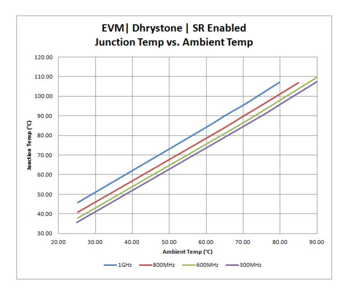
On the EVM baseboard with a worst-case silicon unit, SmartReflex reduces the operating junction temperature by 1-3°C, depending on frequency.
