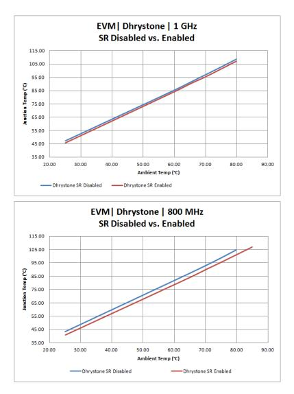
The thermal effect of MPU frequency is significant. At an ambient room temperature of 25°C, the AM335x junction temperature heats up ~10°C while running the Dhrystone application at 300MHz. Operating at 1GHz, the junction temperature increase from ambient is ~22°C! This effect increases as ambient temperature increases.
