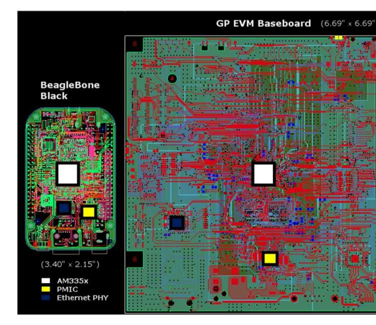
Having over 6 times the board area, the EVM baseboard represents a more thermally effective system solution than the BeagleBone. This means more copper and board space for spreading and dissipating heat. The EVM also has a better component placement in terms of thermal management, as the major sources of heat (processor, PMIC, Ethernet PHY, etc.) are placed spaciously apart on the PCB. The extra room also allows select traces to be wider on the EVM.
