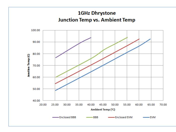
As expected, the enclosed BeagleBone performed the worst and the more thermally-efficient EVM performed the best. The EVM was able to withstand an ambient temperature of 60°C (140°F) before exceeding the 90°C maximum operating junction temperature. However, the enclosed BeagleBone exceeded this at just over 35°C (95°F) ambient.
