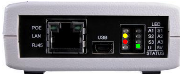
Figure 9 - Bh560v2 End Panel LEDs (normal mode) 1
