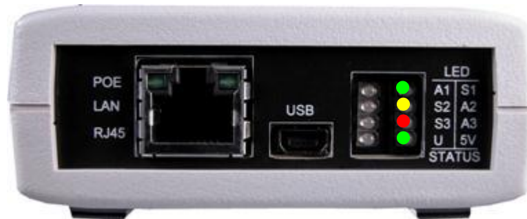
Figure 8- Bh560v2 End Panel LEDs (safe mode) 1
