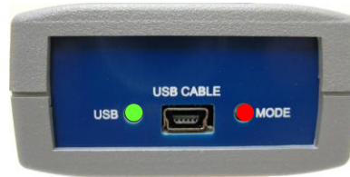
Figure 10 - USB560v2 End Panel LEDs (safe mode) 2
