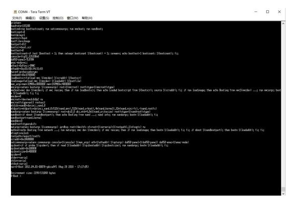
Figure 2 the environment printed from uboot
