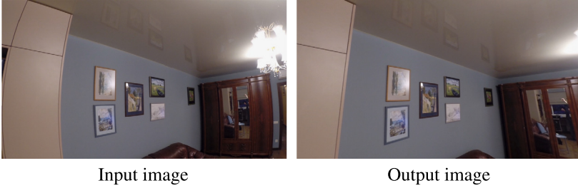
Figure 6.13 Undistort image transformation: input and output. Undistort image transformation: input and output, GoPro HERO 3+, video 1080 p.
