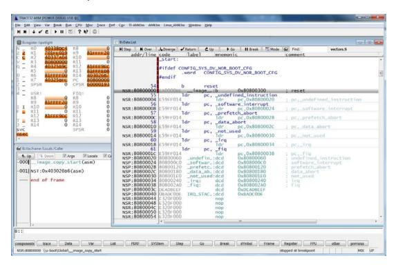
2. At the entry of ENTRY(\_main) in crt0.S for C-runtime startup Code for ARM U-Boot.
