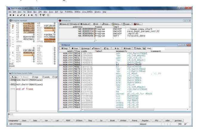
7. Relocate the u-boot symbol using <y.reloc 0x7F729000> for T32 JTAG debugger. The screenshot in #6 is shown below which matches u-boot SRC nicely.
