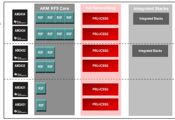
Pin-to-pin and Software Compatible Family of AM2x MCUs
