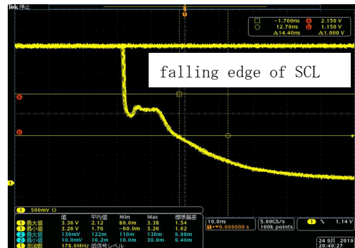
x-axes : 10.0 ns/DIV y-axes : 500 mV/DIV
