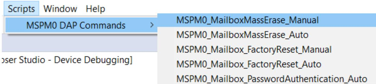
Auto: Means CCS will control the reset pin (Need to connect reset pin to debugger!).
