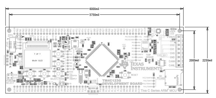
Figure A-1. DK-TM4C123G Component Locations (Top View)
