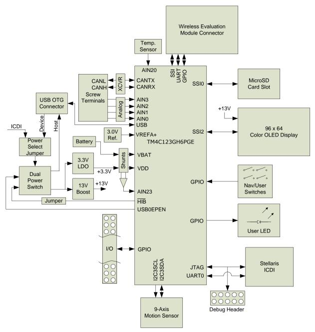
Figure 2-1. DK-TM4C123G Development Board Block Diagram
