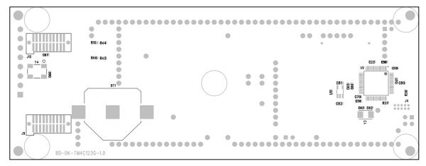
Figure A-2. DK-TM4C123G Component Locations (Bottom View)
