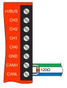
Figure 2-2. Can Diagram
