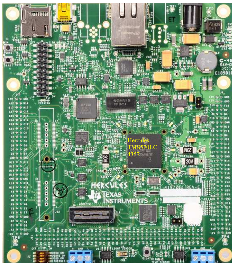
Figure 2-1. TMS570LC43 HDK Board, Interfaces Top Side
