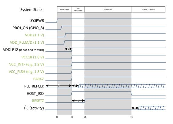
t0: SYSPWR applied to the PMIC. All other voltage rails are derived from SYSPWR
