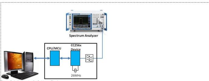
Figure: Typical test setup for Continuous TX mode.
