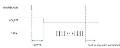
Figure: Device Initialization Sequence
