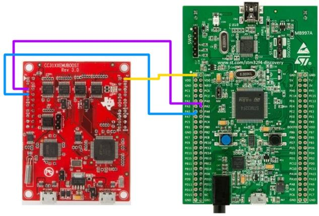
4. Connect the USB cables from the PC to both boards. Mini-USB for STM32F4-Discovery and micro-USB for CC31XXEMUBOOST.
