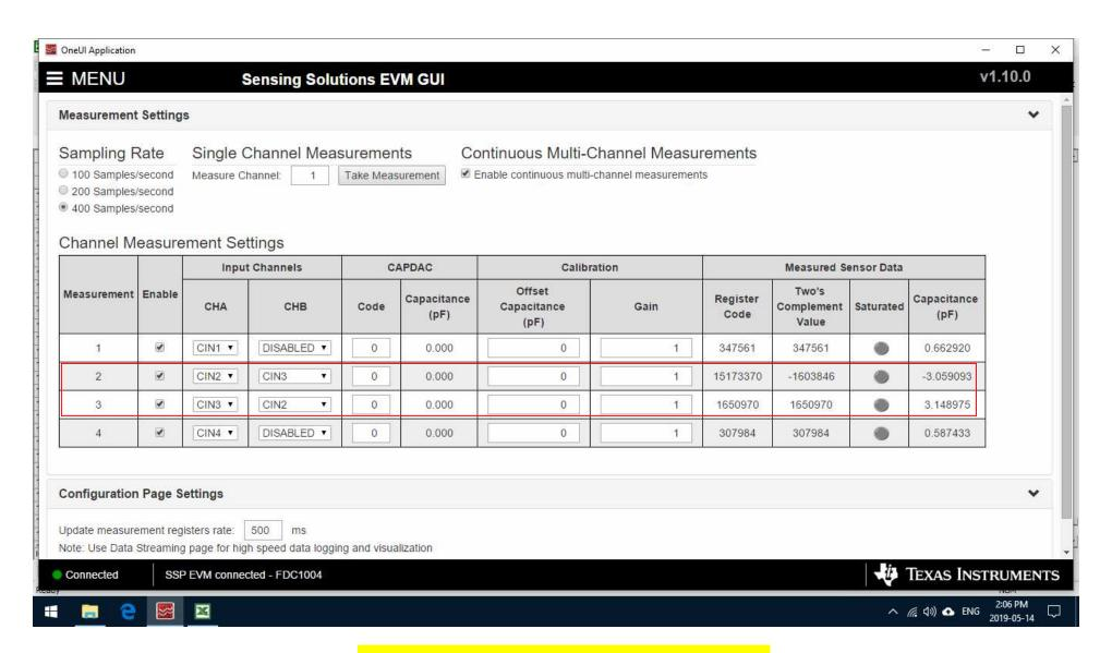
Parallel Plate 1 to Pin J4.7 (CIN3) Parallel Plate 2 to Pin J4.4 (CIN2) No shield on any plate
