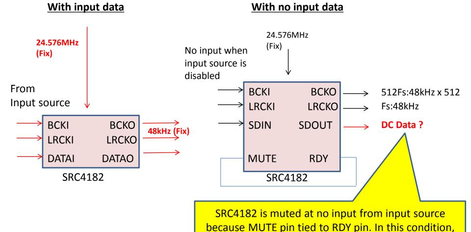
DC level is output from SDOUT and it can cause noise.
