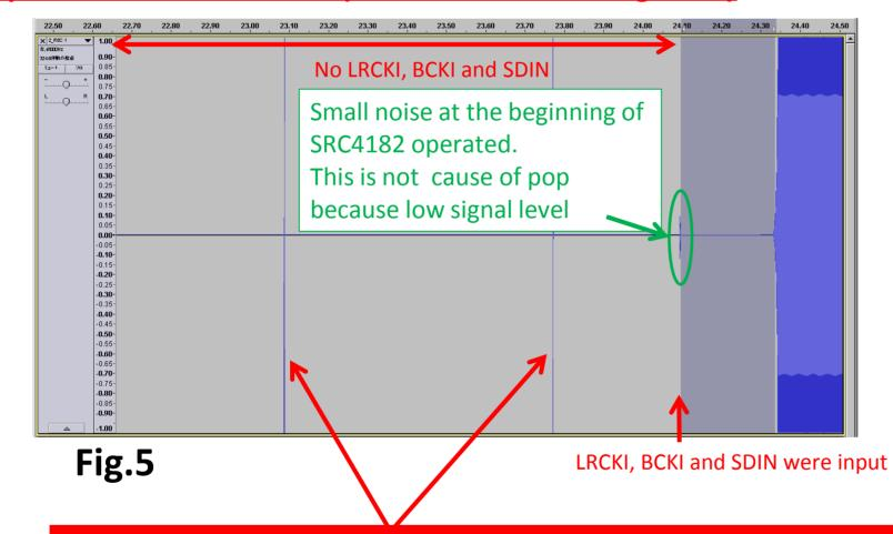
Repeatable signal was output although no SDIN input. This period is 32768Sample (Fs=48kHz).
