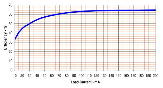
Figure 4: Efficiency over load current
