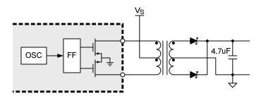
Figure 2: Simplified transformer driver
