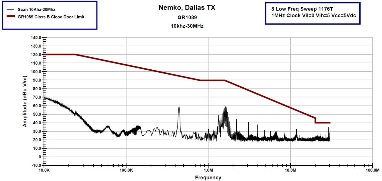
**Figure 3: Radiated emissions (dBuV/m) from 10 kHz to 30 MHz**
