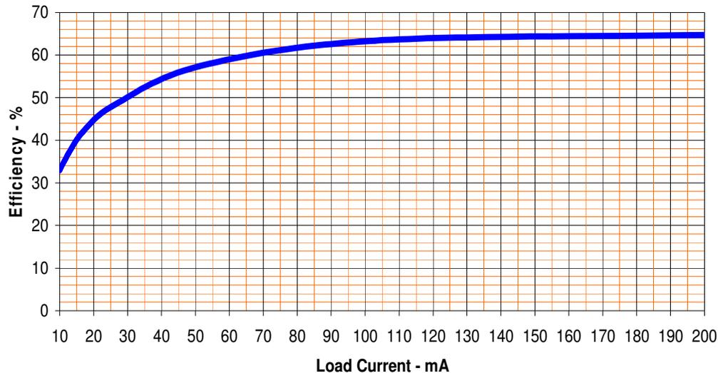
**Figure 4: Efficiency over load current**
