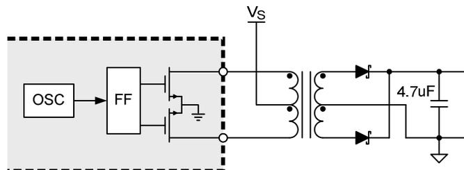
**Figure 2: Simplified transformer driver**
