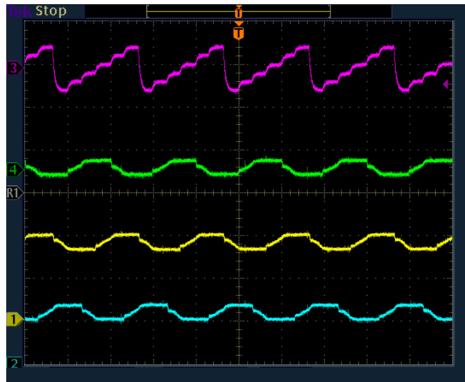
Fig. 19 (a) mod6 counter, (b)BemfA, (c) BemfB (c)BemfC (under 0.5 pu load at 0.3pu speed, Vdcbus=160V)
