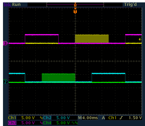
Fig. 10 The PWM outputs , PWM 1 (Yellow) , PWM 2 (Pink) and PWM 5 (Green), PWM 6 (Blue)
