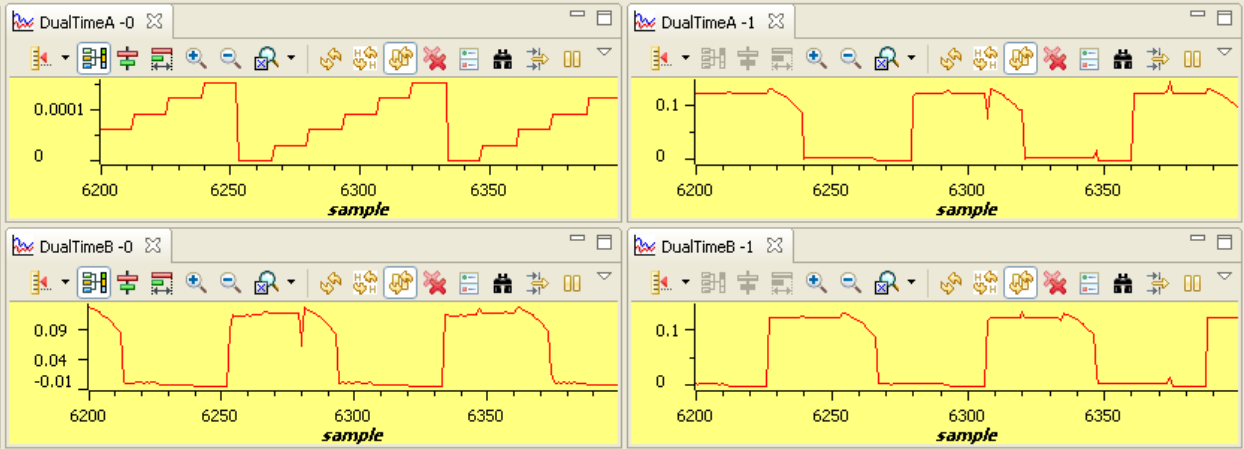
Fig. 14 (a) mod6 counter, (b) BemfA, (c) BemfB and (d) BemfC ( dlog.prescalar=25 and Vdcbus=160V)
