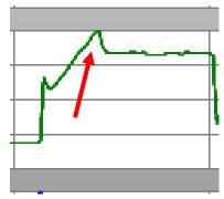
• Adjust the "Flux Threshold" to a smaller value (around 0.4) until the commutation happens right at the inflection point of the voltage waveform.
