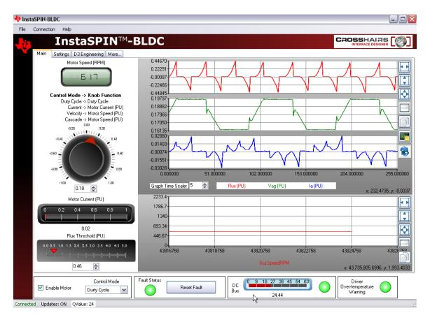
The motor is now tuned for InstaSPIN-BLDC!!!
