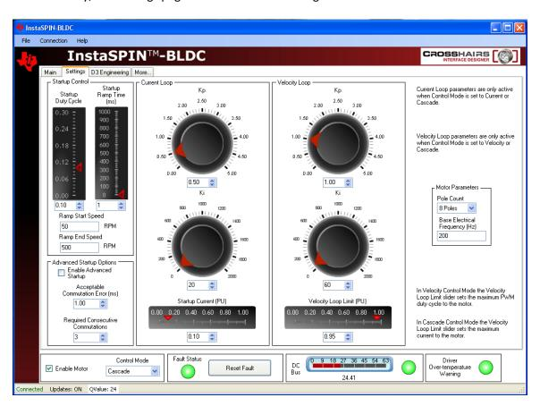
Assuming you haven't changed the Control knob on the "Main" tab, it should still be set to a PU value of 0.3. If not, change it back to that value now. Once again, enable the motor, and verify that it starts up smoothly and achieves a steady state velocity of about 900 RPM.
