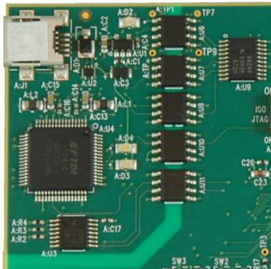
Fig2: xds100v2 Emulation circuitry and isolation circuitry is denoted by an A:
