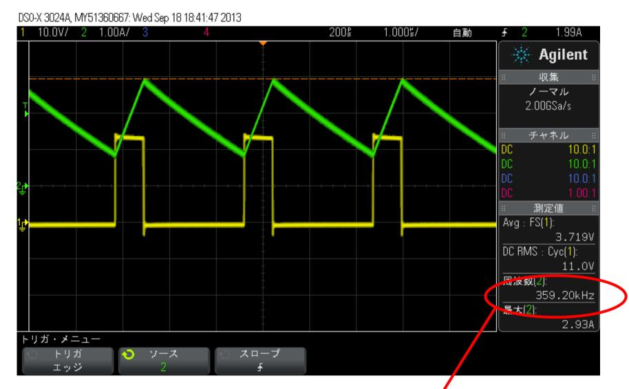
Switching frequency was still 360KHz, and peak inductor current was limited at 3A. If we tried to have more load current, the fsw was folded back as see in next page.
