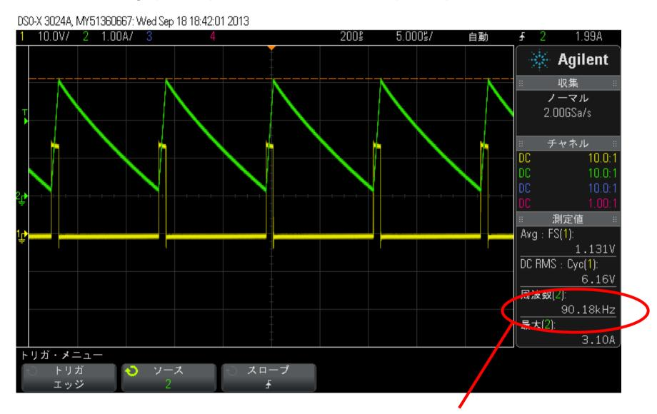
Switching frequency decreased to 90KHz due to the frequency fold back (360/4=90kHz), and peak inductor current was still limited at 3A.
