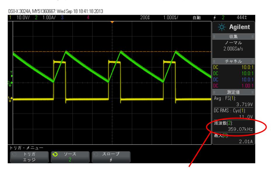
Switching frequency was about 360KHz even though the setting frequency was 720kHz(RT=140k $\Omega$ ).
