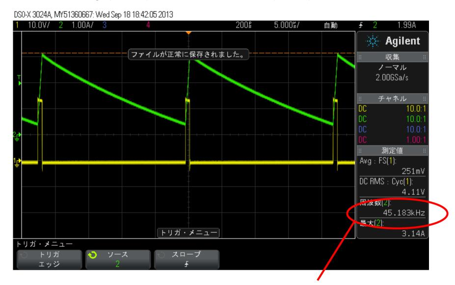
Switching frequency decreased to 90KHz due to the frequency fold back (360/8=45kHz), and peak inductor current was still limited at 3A.
