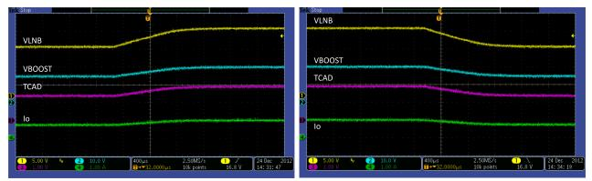
Figure 11. Voltage Transition,  $V_{IN}$  = 12 V, VLNB = 13.4 V to 18.6,  $I_O$  = 1 A
