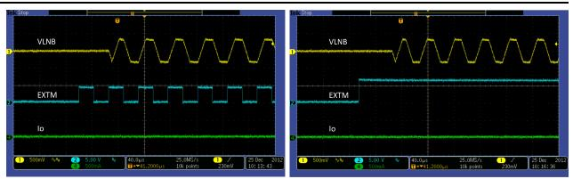
Figure 13. 22-kHz Tone Sync to External Clock,  $\rm V_{IN} = 12~V,~VLNB = 13.4~V,~I_{O} = 0~A$
