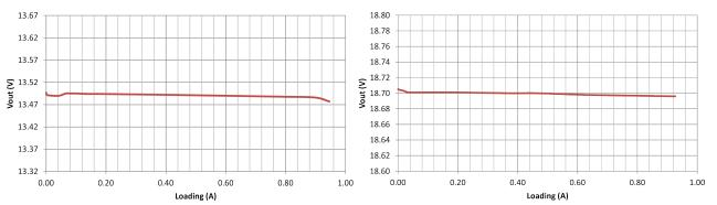
Figure 9. Load Regulation,  $V_{IN} = 12 \text{ V}$ , VLNB = 13.5 V
