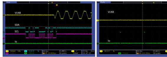
Figure 15. 22-kHz Tone Controlled by  $I^2C$ ,  $V_{\rm IN}$  = 12 V, VLNB = 13.4 V,  $I_{\rm O}$  = 0 A
