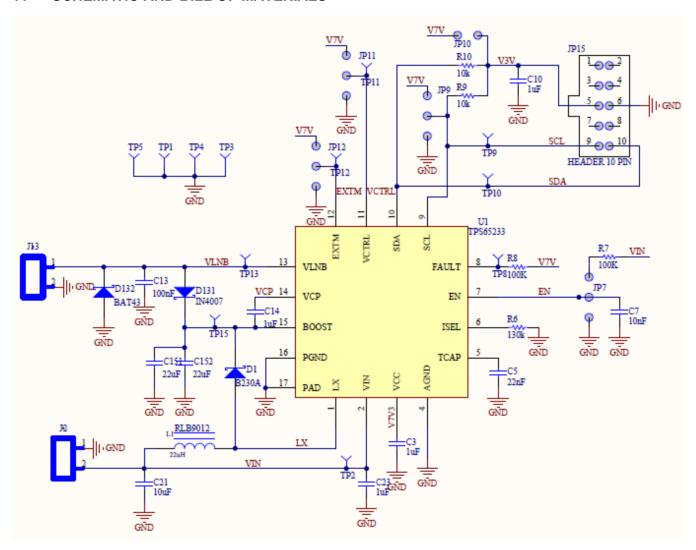
Figure 17. TPS65233EVM Schematic
