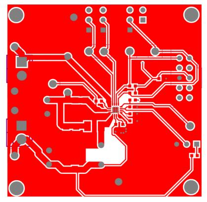
Figure 2. Board Layout (Top Layer)
