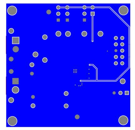
Figure 3. Board Layout (Bottom Layer)
