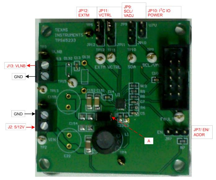
Figure 4. Headers Description and Jumper Placement
