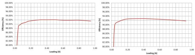
Figure 7. Efficiency,  $V_{IN} = 12 \text{ V}$ , VLNB = 13.5 V
