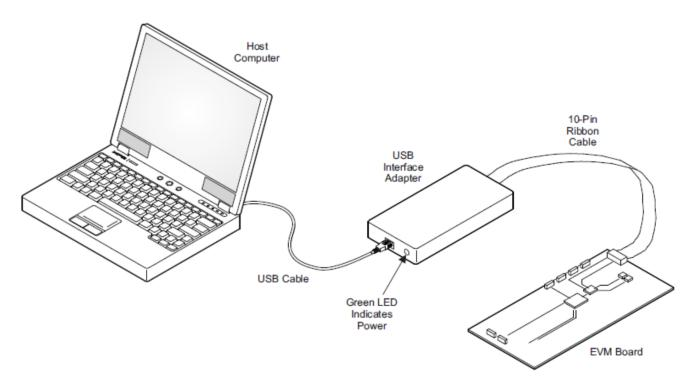
Figure 5. USB Interface Adapter Quick Connection Diagram
