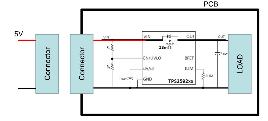
5V is hot-plugged to PCB via connector, then the 5V line may be connected first before GND line connected. Is there any concern or damage to TPS2592xx at this condition?
