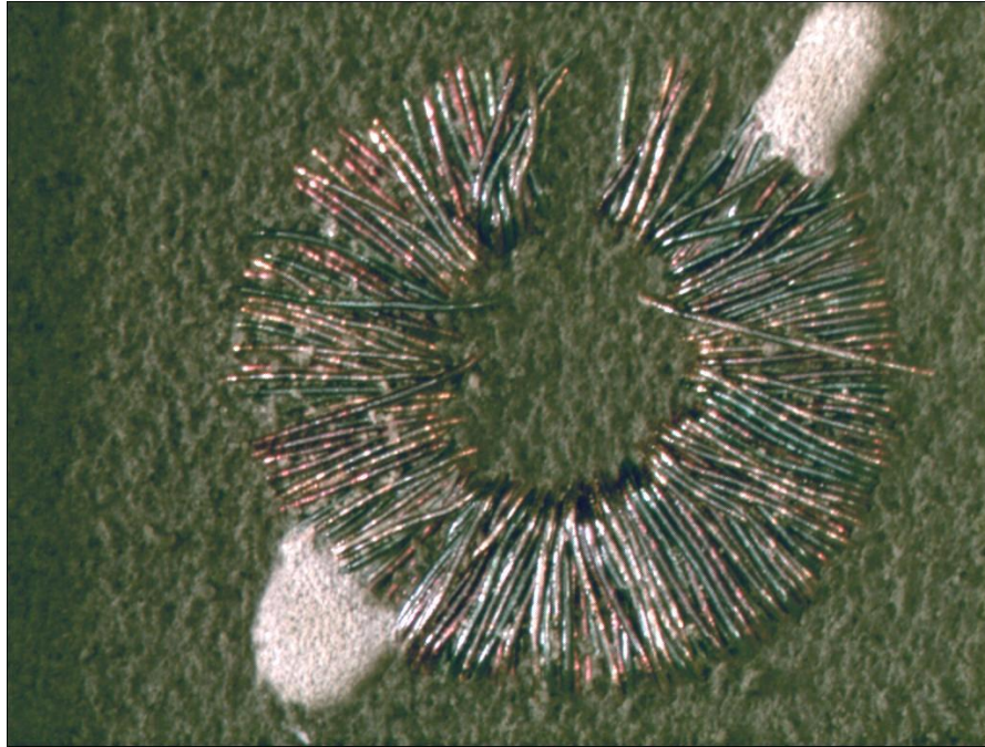
Figure 10. Control Unit. No degraded coating over copper windings is shown.
