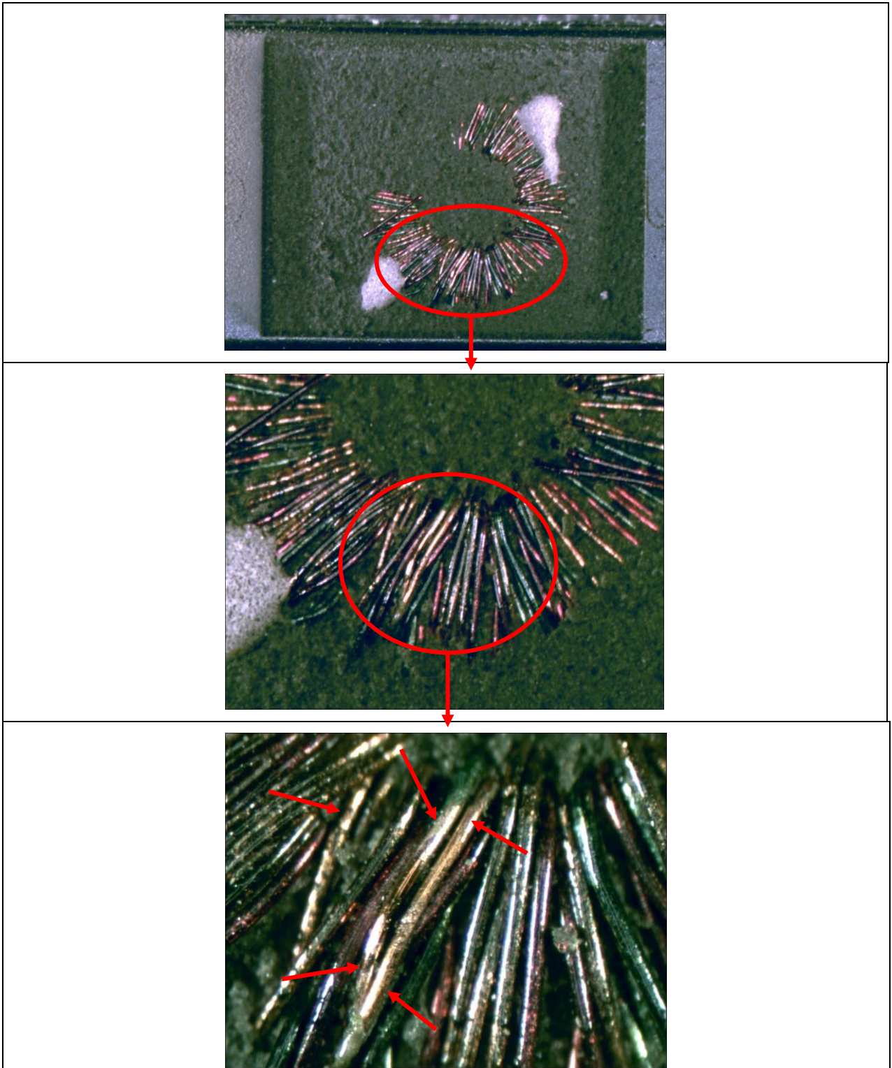
Figure 8. Unit 1. Transformer core windings showed exposed copper.
