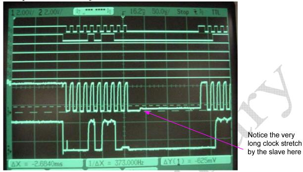
The very long clock stretch here is pretty uncommon but still easily complies with the SMBus specification (25ms packet length). This is a very clean and clear example of a clock stretch. As with this example, most clock stretches happen somewhere around the ACK and NACK clocks.
